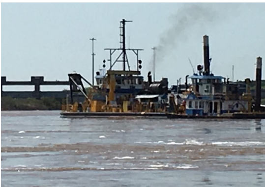
The dredge “Integrity” digging upstream against the current at Lock 1, on the Red R.
