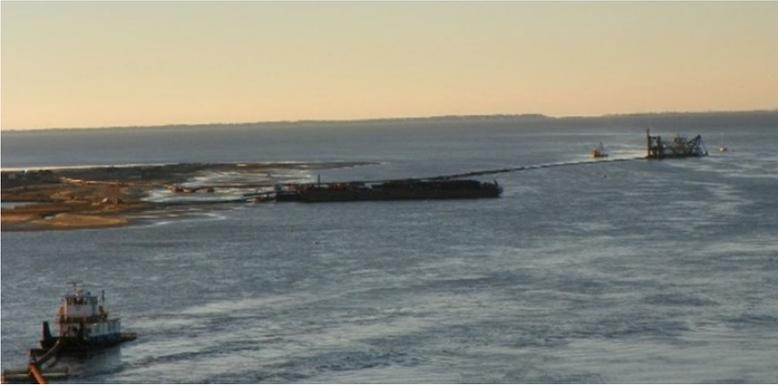
The Ingenuity began the maintenance dredging of the Apalachicola Bay channel in mid December, 2018. The material was pumped onto “Bird Island” at the north end of the bay channel. As the dredge advanced away from the island, line lengths eventually reached nearly 2 miles.
